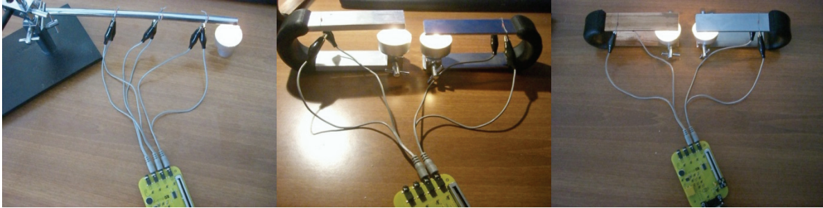
Figure 1. a. The steel bar is heated and three thermistors record its temperature at three different points. b. Two horseshoe aluminum bars with a thickness of 3mm and 8mm respectively are heated and two thermistors record the temperature of each one at some point. c. Two horseshoe bars (a copper one and an aluminum) with a thickness of 3mm are heated and two thermistors record the temperature of each one at some point.
