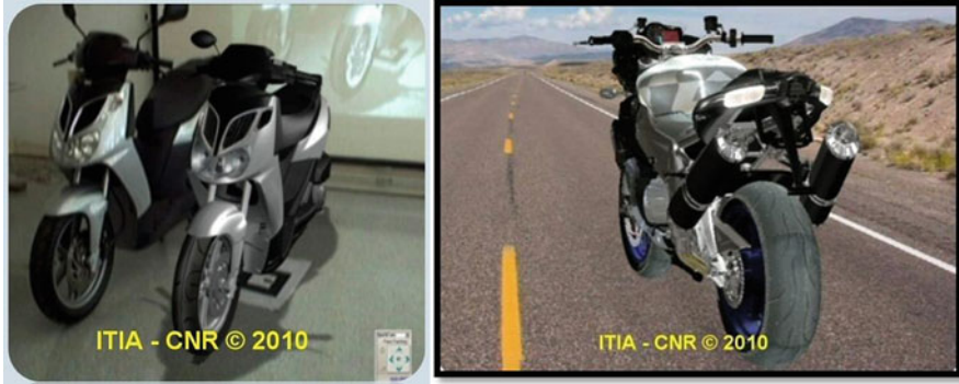
Fig. 1.8 Right picture: Picture of a virtual motorcycle prototype (on the right ) next to a physical motorcycle prototype (on the left ) in the real environment; left picture: virtual prototype in a virtual environment [21]
