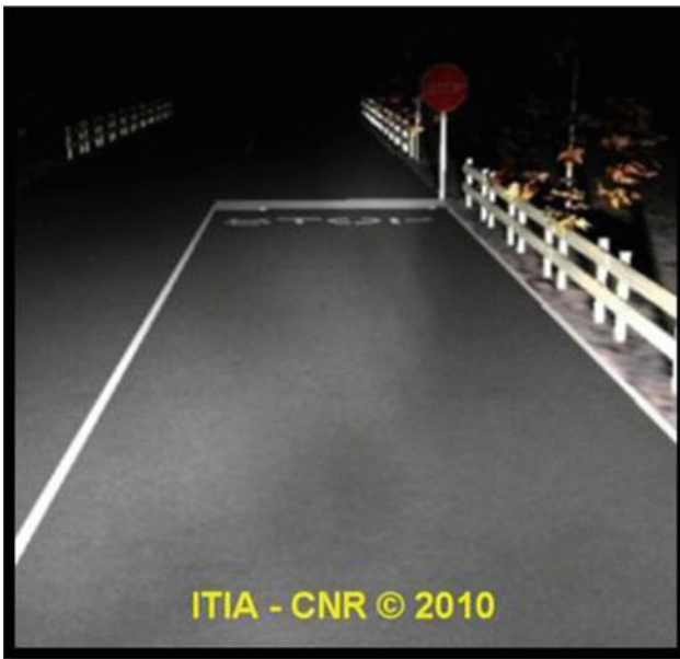
Fig. 1.11 Virtual testing of a lighting system [21]
