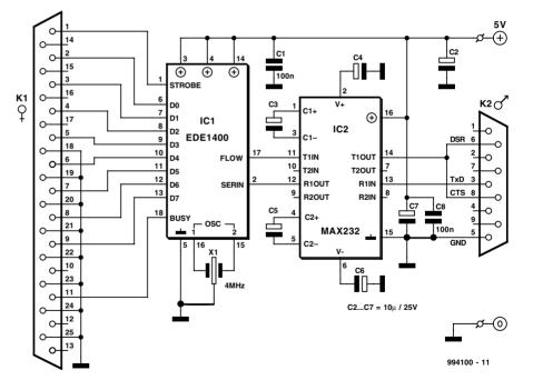
via the Flow signal (pin 17). This ensures that no data is lost. The controller needs a 4 MHz ceramic resonator, X1.
