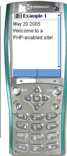
Figure 3: A WML page with dynamic content as displayed through the Openwave Phone Simulator
