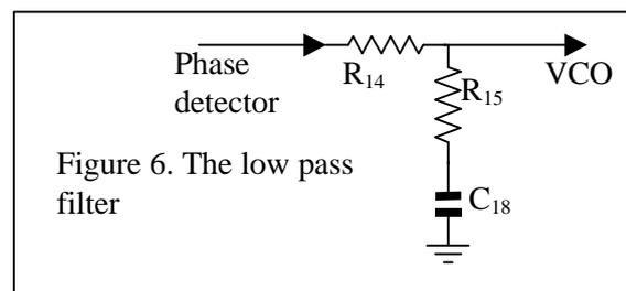
Figure 6. The low pass filter
