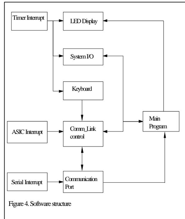
Figure 4. Software structure
