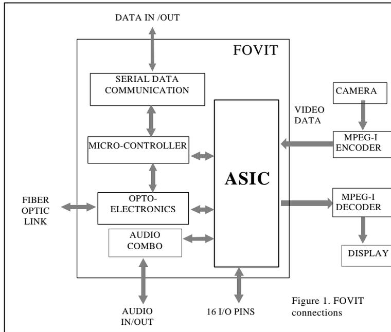
Figure 1. FOVIT connections
