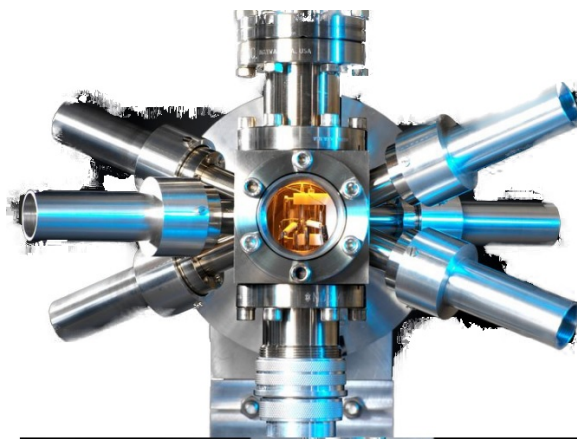
This optical atomic clock uses strontium atoms to tell time. (Npl & Andrew Brookes/Science Photo Library/Corbis)
